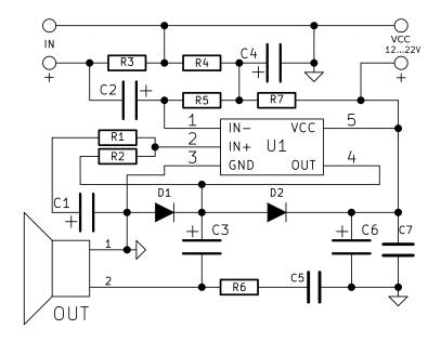
\*We recommend choosing a supply voltage of 12...22Vdc. To obtain more power, replace the standard radiator with a radiator with an effective area of >200 cm2 and replace capacitor C6 with a capacitor for a higher voltage.
