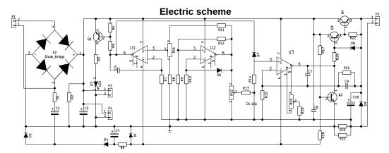
The LPS is a linear power supply with a lownoise element base. The circuit consists of 4 functional units: a reference voltage source, on U2 and D6; a current comparison circuit U1 and RV13; a voltage setting circuit on RV2 and U3.4; a Darlington regulating pair on Q3, Q4 and Q2. When turned on, the U2 microcircuit, which is a type of Schmitt trigger based on an op amp, self-excites due to the positive feedback signal formed by the resistor R12
