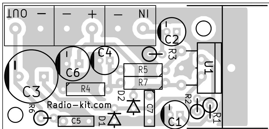
\*We recommend choosing a supply voltage of 12...22Vdc. To obtain more power, replace the standard radiator with a radiator with an effective area of >200 cm<sup>2</sup> and replace capacitor C6 with a capacitor for a higher voltage.
